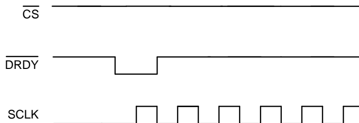
Figure 60. \overline{\text{DRDY}} and SCLK Behavior for SPI Bus Multiplexing
