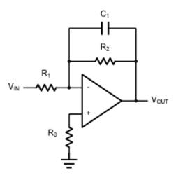
Figure 5. Low Pass Active Filter
