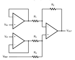
Figure 6. Instrument Amplifier
