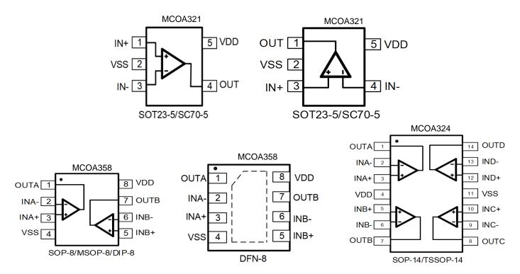
Figure 1. Pin Assignment Diagram
